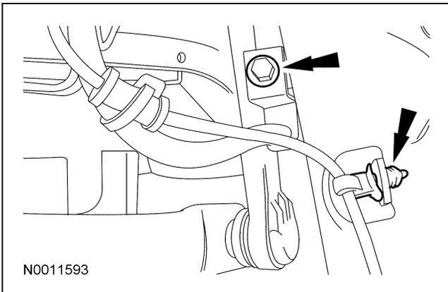
4. **CAUTION:** Support the wheel spindle using mechanic's wire.
