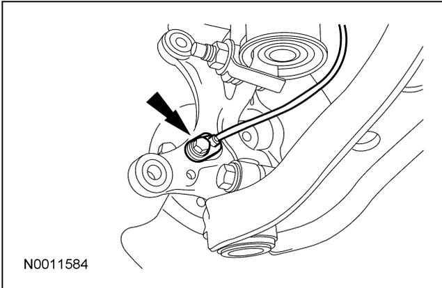
3. Remove the brake line bracket bolt and disconnect the wheel speed sensor wire from the bracket.
