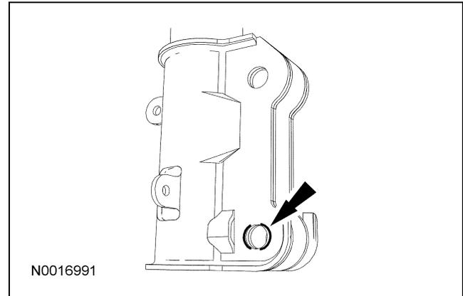
6. **NOTE:** Do not fully tighten the cam bolts until the alignment has been corrected.
